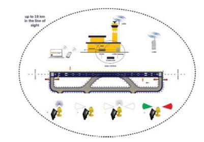
From the POLARIS application the control is more complex. The lights can be controlled individual, in groups, on scenarious and the user can see all the parameters of the lights.
