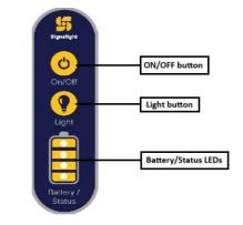
After mechanical installation is done, push the ON/OFF button. This will connect the battery and the POLARIS unit will be powered. As long as the unit is powered the yellow LED from the SIGNALIGHT LOGO will flash every 5 secons. In this moment the lights are in STANDBY mode.
