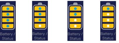
On the second press, the lamp turns on at 1%. With another press, it turns on at 3%, then at 10%, then at 30%, and finally at 100%. If pressed again, the lamp turns off.
