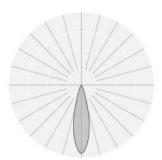
Fixture luminous flux:2320lmFixture luminous efficacy:116lm/WOptical distribution:symmetrical
