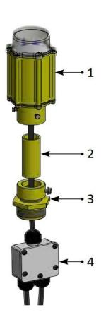
1.Light Flxture pre cabled with 0,5m cable
